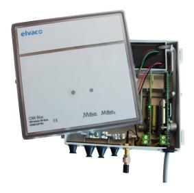
CMi5110 is a wireless M-Bus Receiver, integrated in a CMi-Box, which can be used by any existing wired M-Bus solution or together with Elvaco CMe Series products. CMi5110 communicates with meters via the wireless modes S1, T1 and C1, and is compatible with all widely used wireless M-Bus meters on the market. The product handles up to 800 meters, which can be individually secured by encryption keys.
