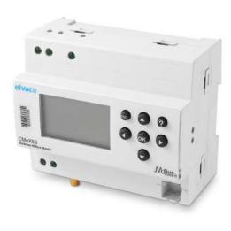
CMeX50 is a wireless M-Bus Receiver which can be easily integrated into an existing M-Bus solution or used together with Elvaco CMe Series products. The CMeX50 communicates with up to 800 wireless M-Bus meters, each one securable through individual encryption keys. CMeX50 also has an integrated M-Bus Master which enables it to drive up to 32 wired M-Bus meters. The number can be extended by using the product together with one of Elvaco's M-Bus Masters from the CMeX10-13S Series.
