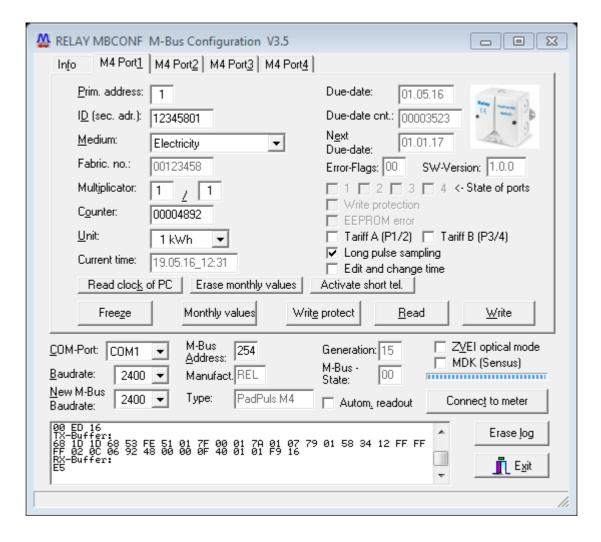
This sheet shows the current settings and values of the respectively pulse channel (port) of the PadPuls M2C/M4C (in this example: M4C Port 1 in the mode "long telegram"). The following input boxes and buttons are used to change the parameters of the pulse adapter:
