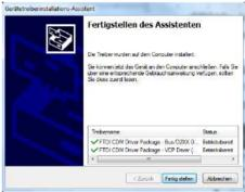
Now you can connect the PC. The USB driver for the PW250 is installed automatically and generates a new, virtual COM port. The new Comport number of the USB serial port is displayed after completion of the installation (here: COM29). You can look up this number at any time in the Device Manager under ports (USB Serial Port) and - if desired – change it in the advanced settings of the driver. Please select the appropriate comport number in your M-Bus software.
