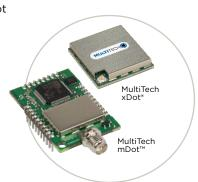
The mDot and xDot are LoRaWAN compliant,
