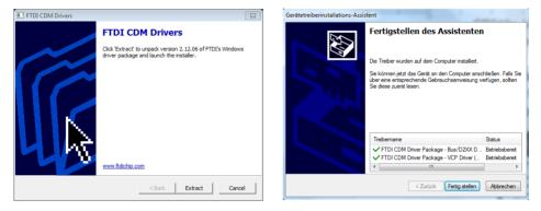
Now you can connect the PC. The USB driver for the PW100 is installed automatically and generates a new, virtual COM port. The new COM port number of the USB serial port is displayed after the installation is finished (here: COM29). You can look up this number at any time in the Device Manager under ports (USB Serial Port) and - if desired – change it in the advanced settings of the driver. Please select the appropriate comport number in your M-Bus software.
